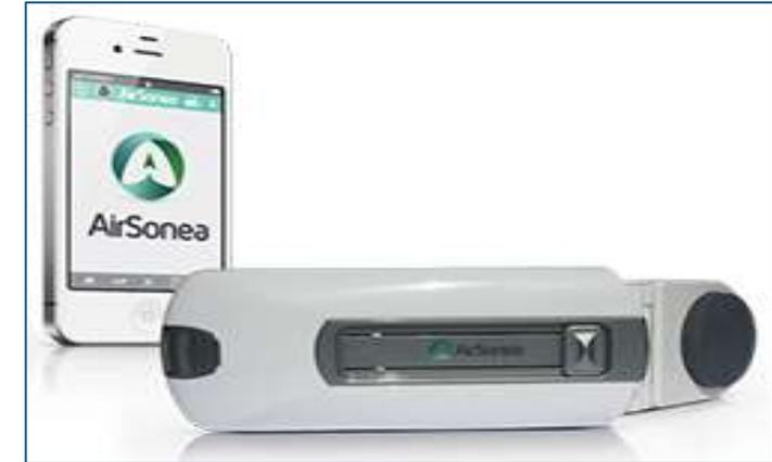
The AirSonea device, which connects to an asthma patient's smartphone and communicates with wheeze analysis algorithms on iSonea's server.
